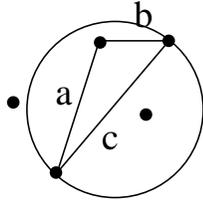
**Figure 2: Communication on an edge  $c$  is more expensive with regard to unit energy than communication on the edges  $a$  and  $b$  ( $a^2 + b^2 < c^2$ )**
