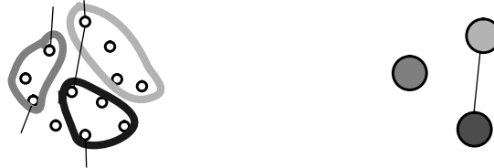
Figure 16. Nodes covered by matches of distinct patterns with match graph, denoting their dependency
